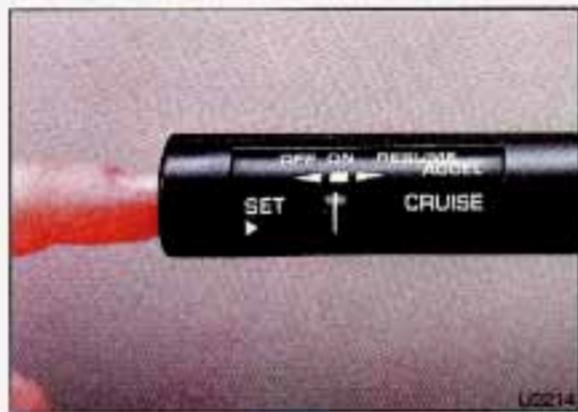
3. Push in the **SET** button at the end of the lever and release it.
