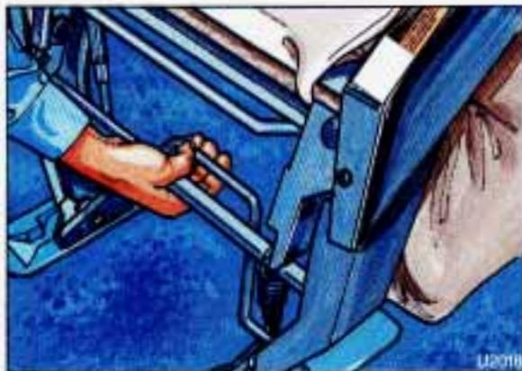
3. Then, from behind the seat, support the top portion of the seat with one hand as you squeeze the front release bar toward the crossbar. The seat will release from the floor pins.
