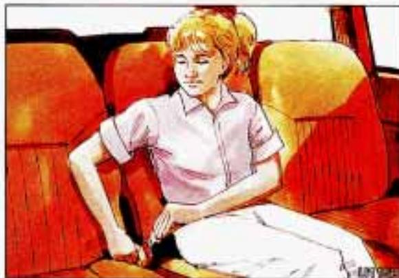
1. Pick up the latch plate and, in a single motion, pull the belt across you. Don't let it get twisted.
