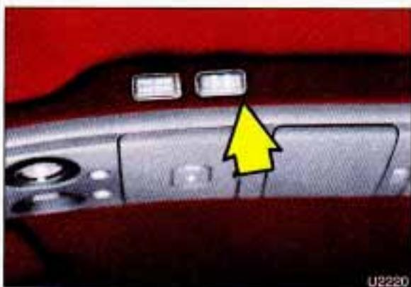
The sliding door must be unlocked for the power sliding door to operate. The key does not have to be in the ignition. To help avoid accidental operation of the sliding door, disable the power sliding door by placing the power sliding door override switch in the **OFF** position.
