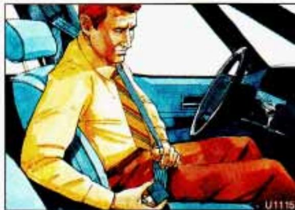
If the belt stops before it reaches the buckle, tilt the latch plate and keep pulling until you can buckle the belt. If the belt isn't long enough, see the *Index* under *Safety Belt Extender*.
