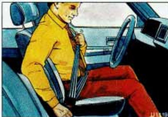
5. To make the lap part tight, pull down on the buckle end of the belt as you pull up on the shoulder belt.
