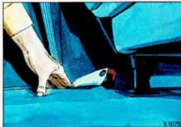
Anchor brackets for the second row outside positions are located just above the place where the third row lap-shoulder belts meet the floor. There's a vinyl sleeve there; to get to the bracket, push this vinyl sleeve aside slightly. Anchor the top strap to the bracket.
