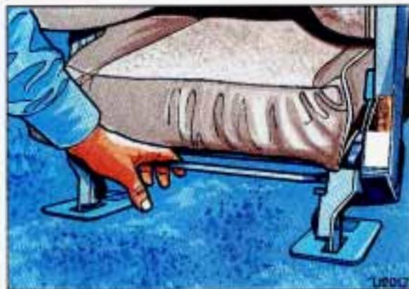
2. Push down on the rear release bar. The entire seat will tilt forward.
