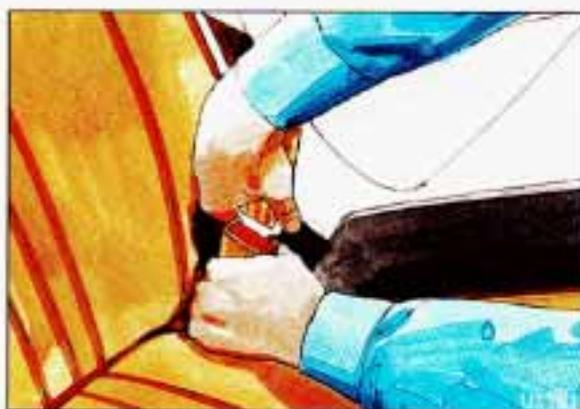
4. While holding it out, run the belt through or around the child restraint. The child restraint instructions will show you how.
