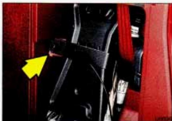
2. Remove the jack and jacking tools by loosening the wing nut and retainer bar.
