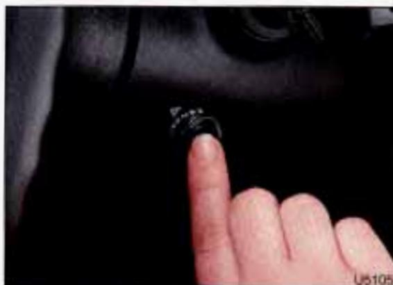
Your hazard warning flashers switch is on the steering column below the ignition switch. Press the button in to make your front and rear turn signal lights flash on and off.
