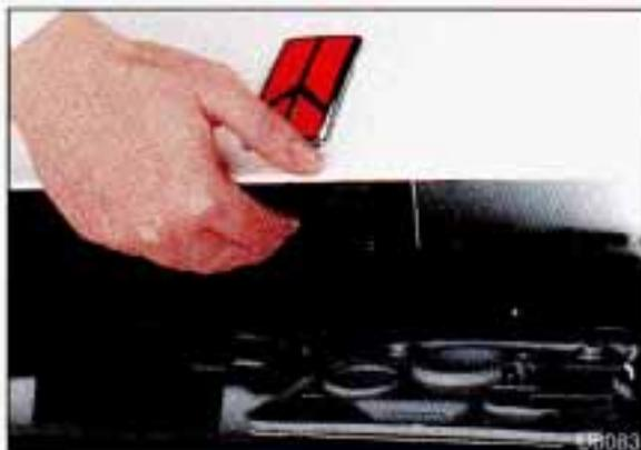
Then go to the front of the vehicle and pull up on the underhood release. Lift the hood.
