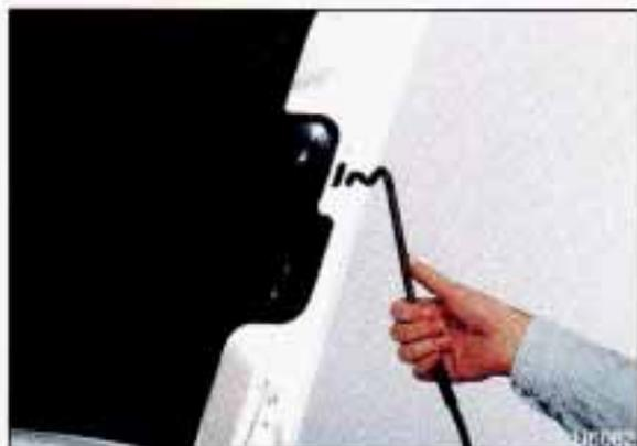
The hood prop rod may be hot due to increased engine temperatures under the hood, so be careful when handling it. Use your hood prop sleeve when handling the prop.
