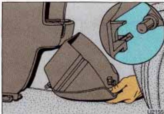
To replace the bin, set the hinge pins (one on each side of the bin, at the bottom) into the hinge guides (one at each side of the console opening, at the base), then close the bin. If the hinge pins are placed properly in the guides, the bin will close easily.
