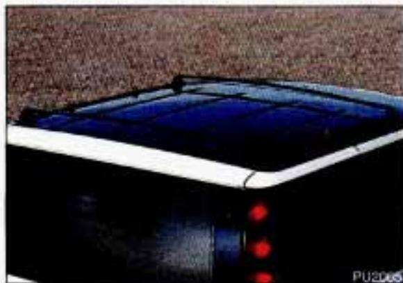
The side of the convenience net closest to the front of the vehicle is higher than the side closest to the liftgate. Once you've loaded items into the net, stretch the higher side of the net up and over the top of the load to hold it firmly in place.
