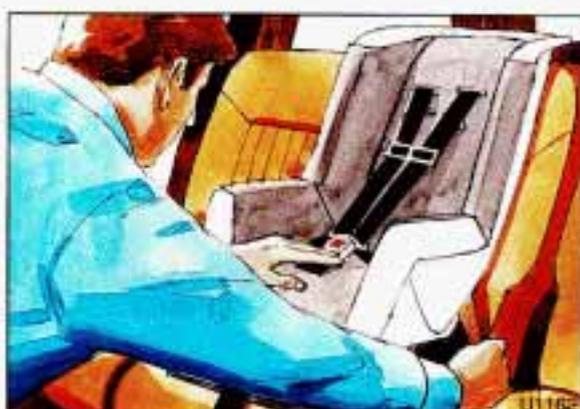
6. To tighten the belt, feed it back into the retractor while you push down on the child restraint.
